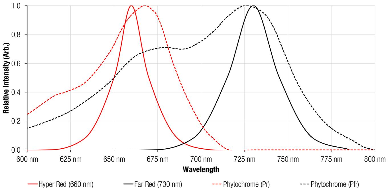
Figure 5: The absorption spectra of phytochromes Pr and Pfr and the light output of the WL-SMDC hyper-red ([150353HS74500](#)) and far-red ([150353FS74500](#)) Ceramic LEDs
